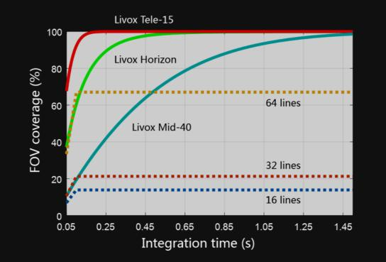
Fig.3 The FOV coverage of Livox LiDAR sensors, including Horizon, Tele-15, and Mid-40; compared with other (non-Livox) LiDAR sensors that used common mechanical scanning methods, with linenumber and vertical FOV being 64 lines/27°, 32 lines/41°, 16 lines/30°. During calculation, the FOV is gridded with 5mrad\*5mrad.
