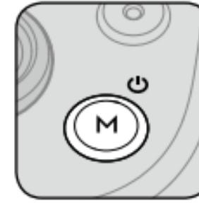
When powered off, press once to check battery level. Press and hold to power on or off.
