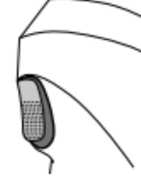
Press and hold to enter lock mode, and release to exit lock mode.
