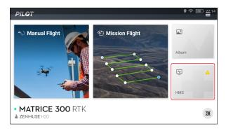
2. The health condition of each module of the connected device will be displayed onscreen.
