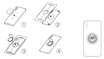
2. Align the marks on the phone clamp or ring holder and the mounting plate. Attach the mobile phone to DJI OM 4.
