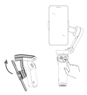
Mount your mobile phone before powering on DJI OM 4. If no mobile phone is detected, DJI OM 4 will vibrate and enter standby mode. To bring it out of standby mode, press any button after mounting the mobile phone.
